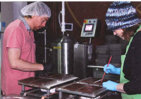
Paul and Candi move chocolate into the corners of the chocolate bar mold while it's on a shaker, assuring consistent dosing and even chocolate throughout the bar.
