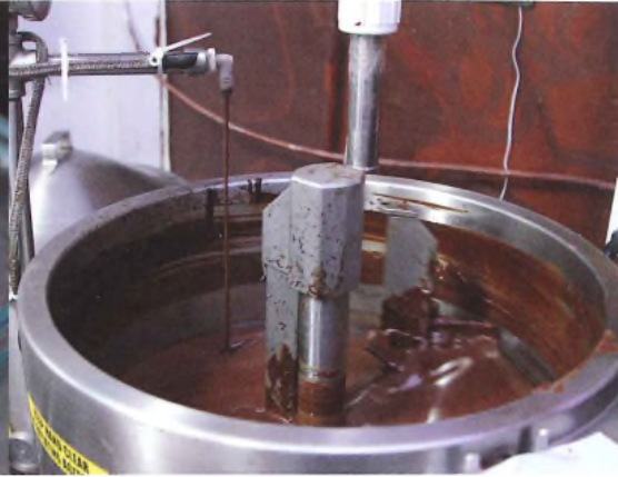
Automated tempering machine heating, stirring, and circulating the melted chocolate.
